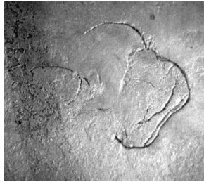
Fig. 1. Typical of cold-flow surface defect [2]
