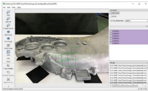
Fig. 7. Annotation process using labelImg by tzutalin
