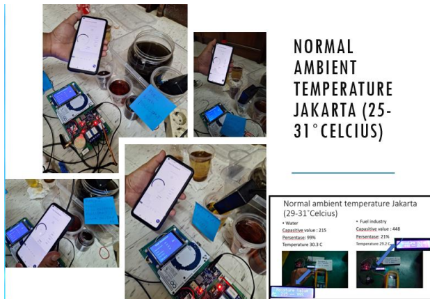
Fig. 7. Experiment with capacitive soil moisture sensor
