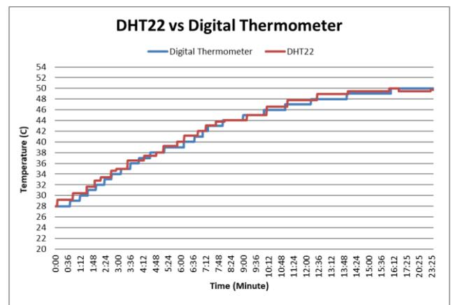
Fig. 6. The comparison of reading temperature result between DHT22 sensor and krisbow digital thermometer
