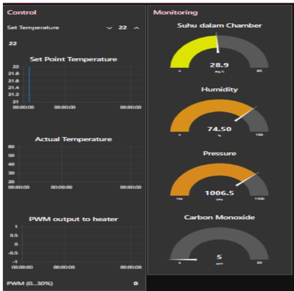
Fig. 7. Dashboard of ETC monitoring system in webserver
