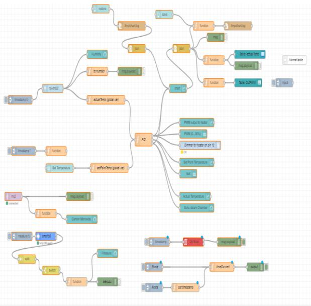
Fig. 4. Flow Program ETC in application Node red
