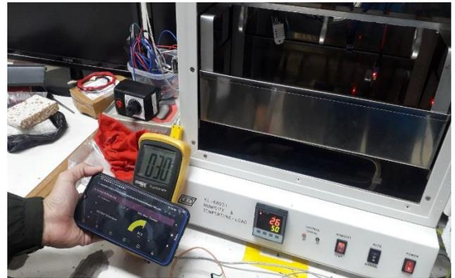
Fig. 5. The comparison of temperature measurement of DHT22 sensor and krisbow digital thermometer
