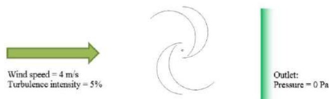
Figure 10. Simulation conditions for 2 different attitude of VAWT turbine.
