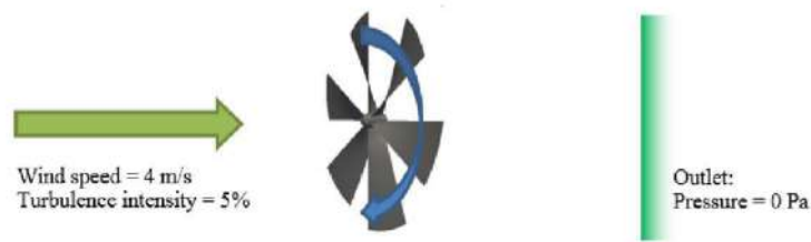
Figure 6. Simulation boundary conditions for turbine CFD analysis.
